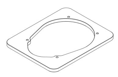
**Note:** Mount Sensor Shield using M6x1 threaded holes, as located in plate above. (Cut pattern available upon request).
