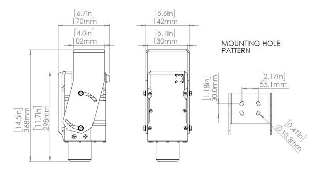
**Note:** Mounting bracket with dampers available for extreme vibration environments such as hard-rock drilling rigs and continuous miners.
